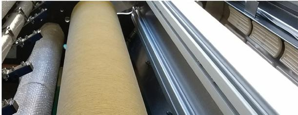
This micro-perforator is designed to punch **MICRO HOLES** in moving film using **HOT NEEDLES**. This machine has to be integrated into existing machinery such as extruders, bag machines, slitters or printing machines. The **HN100** is a **MOTORIZED**
